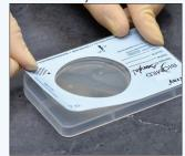
Reseal the InTray label to the plastic tray body. Press all around the perimeter of the InTray to ensure a complete seal.
